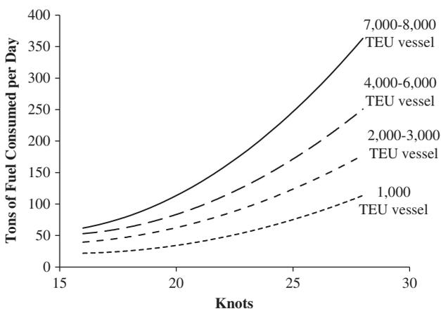
**Figure 1:** Container ship fuel consumption by vessel size.
